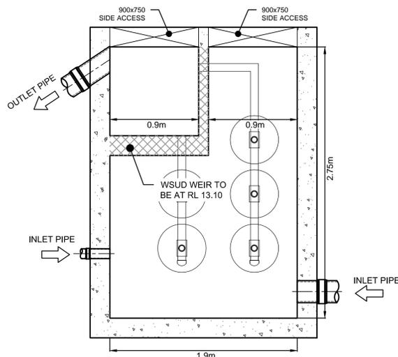
**UNDERGROUND OSD/WSUD TANK DETAIL PLAN VIEW**
